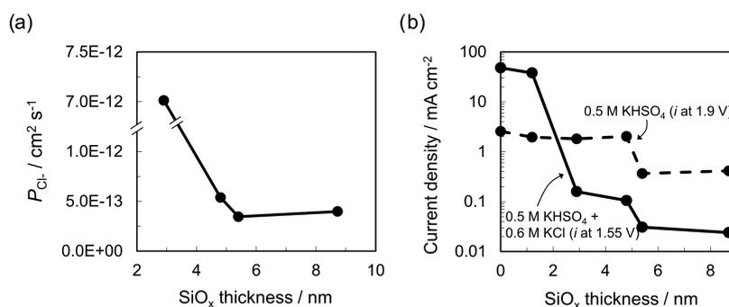
**Figure 4.** (a) Permeability of Cl<sup>-</sup> in SiO<sub>x</sub> overlayers as a function of overlayer thickness, calculated from LSVs for SiO<sub>x</sub>|Pt in 0.5 M KHSO<sub>4</sub> + 0.6 M KCl using eq 4. (b) Current densities for SiO<sub>x</sub>|Pt recorded at +1.90 V vs RHE during LSVs in 0.5 M KHSO<sub>4</sub> (dashed curve) and recorded at +1.55 V vs RHE during LSVs in 0.5 M KHSO<sub>4</sub> + 0.6 M KCl (solid curve).
