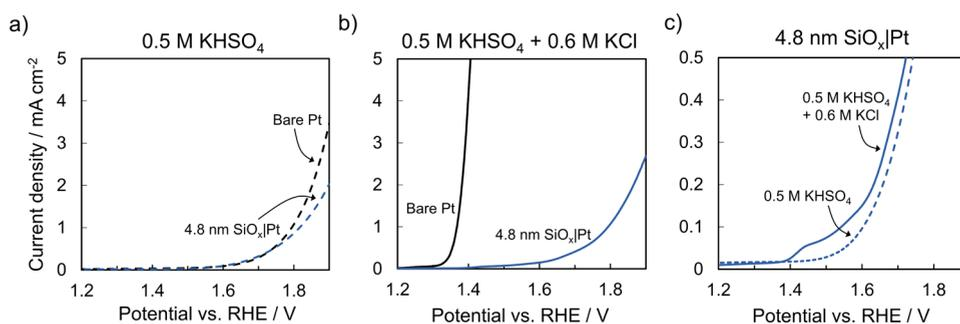
**Figure 3.** LSV measurements for bare Pt and  $\text{SiO}_x|\text{Pt}$  electrodes in (a) 0.5 M  $\text{KHSO}_4$  and (b) 0.5 M  $\text{KHSO}_4 + 0.6$  M  $\text{KCl}$ . (c) LSVs for 4.8 nm  $\text{SiO}_x|\text{Pt}$  in 0.5 M  $\text{KHSO}_4$  and 0.5 M  $\text{KHSO}_4 + 0.6$  M  $\text{KCl}$  (order-of-magnitude shorter vertical axis). All measurements were performed at 20  $\text{mV s}^{-1}$  in deaerated electrolyte at pH 0.8 and 25  $^\circ\text{C}$ .
