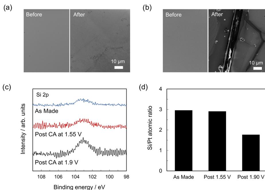
**Figure 6.** SEM images of 4.8 nm SiO<sub>x</sub>/Pt before (left) and after (right) 12 h CA in 0.5 M KHSO<sub>4</sub> + 0.6 M KCl at (a) 1.55 V vs RHE and (b) 1.90 V vs RHE. (c) XPS Si 2p spectra for 4.8 nm SiO<sub>x</sub>/Pt electrodes as-made and post-CA and (d) Si/Pt atomic ratio for as-made and post-CA samples. CAs performed in 0.5 M KHSO<sub>4</sub> + 0.6 M KCl electrolyte for a duration of 12 h. Potentials provided in the subfigures are given vs the RHE.
