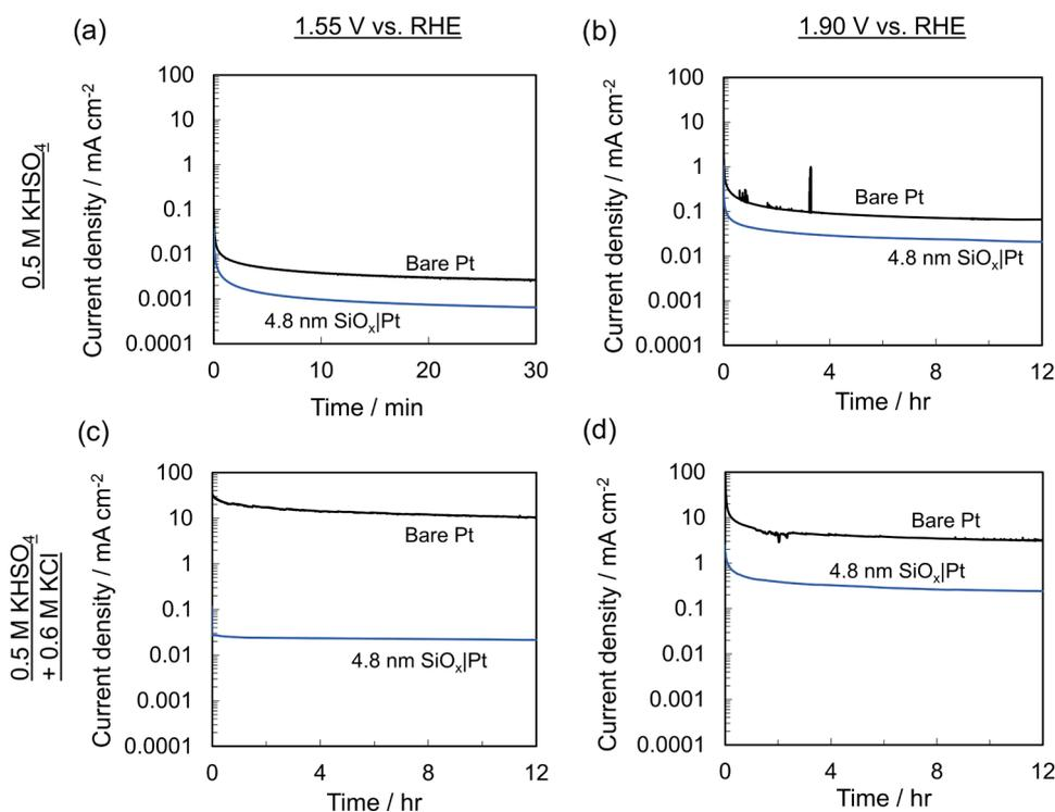
**Figure 5.** CA stability measurements for bare Pt and 4.8 nm SiO<sub>x</sub>|Pt in 0.5 M KHSO<sub>4</sub> at constant applied potentials of (a) 1.55 V vs RHE and (b) 1.90 V vs RHE. 12 h CA stability measurements for bare Pt and 4.8 nm SiO<sub>x</sub>|Pt in 0.5 M KHSO<sub>4</sub> + 0.6 M KCl at constant applied potentials of (c) 1.55 V vs RHE and (d) 1.90 V vs RHE. All measurements were performed in deaerated electrolyte at pH 0.8 and 25 °C.
