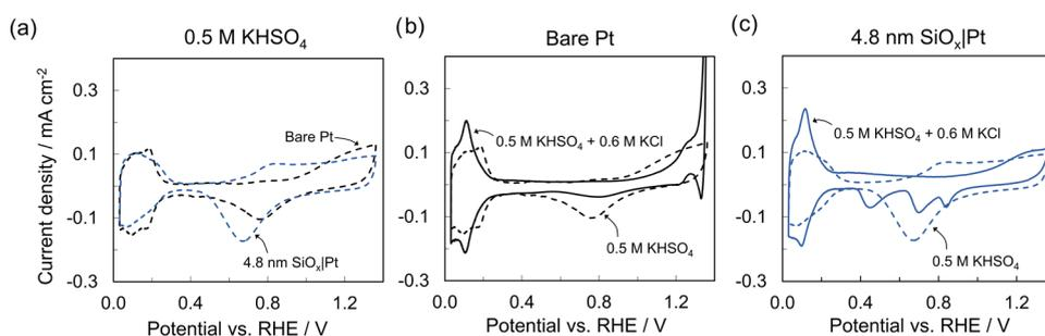
**Figure 2.** CV measurements for (a) bare Pt (black curves) and 4.8 nm SiO<sub>x</sub>|Pt (blue curves) in 0.5 M KHSO<sub>4</sub>. CV measurements for (b) bare Pt and (c) 4.8 nm SiO<sub>x</sub>|Pt in 0.5 M KHSO<sub>4</sub> (dashed curves) and 0.5 M KHSO<sub>4</sub> + 0.6 M KCl (solid curves). All measurements were performed at 100 mV s<sup>-1</sup> in deaerated electrolyte at pH 0.8 and 25 °C.
